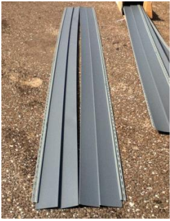
*Bow – panels touch at middle, ends flair
